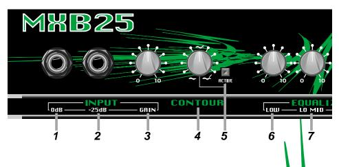
**1: 0dB INPUT:** Use this 1/4" jack to connect your instrument to the amplifier by means of a shielded instrument cable. If your instrument has active electronics or high output pickups, or if the amplifier distorts at low settings of the Gain control (#3), use the -15dB Input jack (#2).
